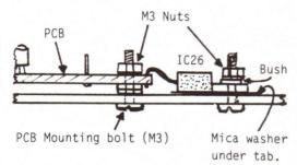
The display module runs quite warm. Ensure that heat from the module does not warm up any associated VFO circuitry. Heating a VFO will lead to unwanted frequency drift.
