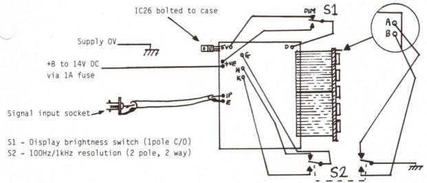
The diagram shows the DFD5 wired for general purpose use in its own case. If it is to be built into a receiver etc, then you may choose to "hard wire" the kHz/100Hz selection instead of fitting a switch. The normal/dim selection could also be hardwired rather than switched.
